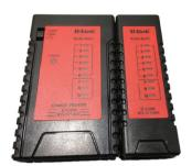
The D-Link LAN Tester can be used for testing RJ45 cables, RJ11 telephone cables and network cables. It keeps your network running smoothly by testing wrong connection, short circuit and open circuit, the two-part unit can be separated for remote closet testing.
